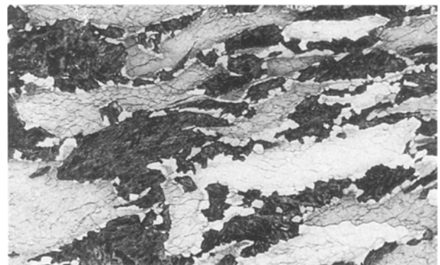
Figure 2 Optical micrograph showing fibrous martensite and substructure in ferrite, specimen 50BQ780 × 1560.
